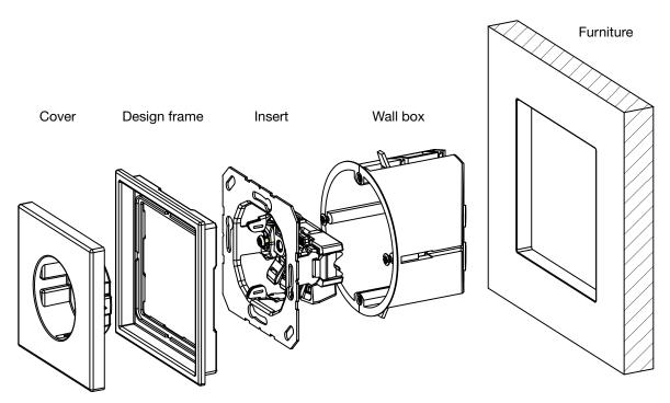
The flush mounting installation requires a minimum panel thickness of 13 mm. The supporting frame contact surface must be generated smooth and flat. Subsequently the cut out has to be sealed with a suitable sealing in order to avoid a swelling of the furniture.
