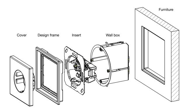
The flush mounting installation requires a minimum panel thickness of 13 mm. The supporting frame contact surface must be generated smooth and flat. Subsequently the cut out has to be sealed with a suitable sealing in order to avoid a swelling of the furniture.
