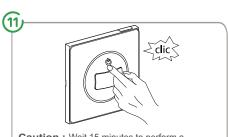
**Caution:** Wait 15 minutes to perform a functional test. Walk through the detection area and make sure the load is activated: light on, motor on.
